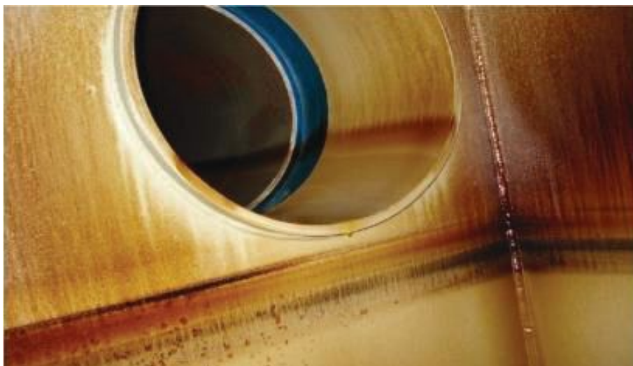
Figure 2 | Since polar compounds are attracted to one another, degraded lubricants can have a greater affinity toward metal turbine parts, where they will collect as varnish. (Figure courtesy of Fluitec.)
