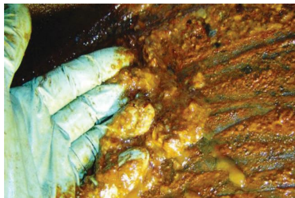
Figure 3 | When large quantities of varnish accumulate in the oil, they begin to precipitate out of solution into a thick gooey layer of sludge. (Figure courtesy of Greg Livingstone and Fluitec.)
